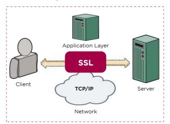
**Network** - TCP/IP facilitates the delivery of network packets between network points. TCP/IP is a peer to peer protocol (e.g. a client connects to a server). The life of such a connection is determined by the duration of the particular exchange.
